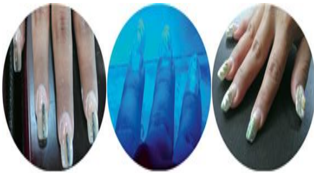
Fig2: Prototyping beauty tech nails. Gel nail process. Step 1. RFID tag placed on the top of the dried basecoat gel, Step 2. curing gel layers, Step 3. decorative nail design.
