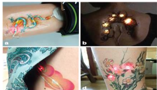
Fig6: Example of skintillates tattoo displays. (a) a dragon skintillates display is powered by the watch and could serve as a point-light display, (b) a back skintillates tattoo that flashes with the beat of the
