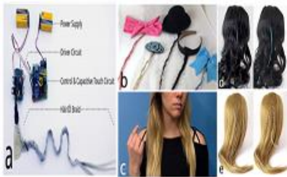
Fig10: (a) HäirIÖ prototype before miniaturization, (b) exemplar HäirIÖ hair accessory form factors, (c) HäirIÖ uses Swept Frequency Capacitive Sensing to detect natural hair interactions, (d) HäirIÖ color-changing properties using thermochromic pigments, and (e) shape-changing properties using Nitinol wire
