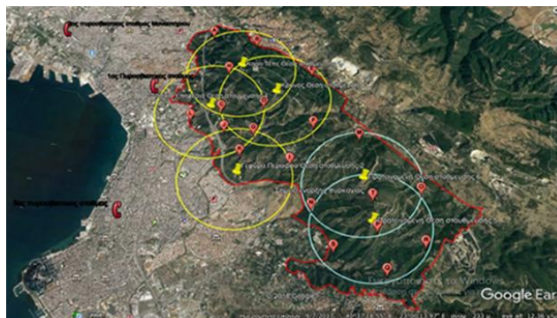
Figure 3. Google map of research area and a 1.5 km radius centered forest fire observation sites for immediate extinguishment within 10' to 15'. The yellow cycles are the ones where Fire Department is pointed four 4X4 firefighting vehicles. The blue radius are the ones that are proposed after our research.
