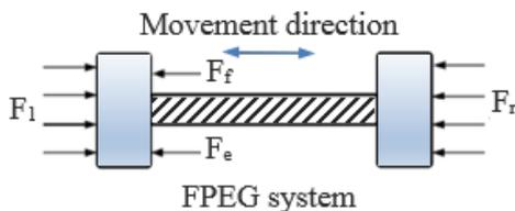
Fig-3: Forces applied over piston-connecting rod mechanism
