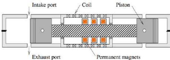
Fig-2: Illustration of the free-piston engine generator
