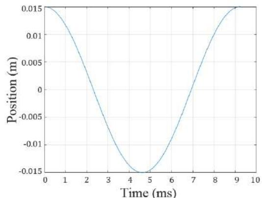
Fig-4: Conventional ICE piston dynamics
