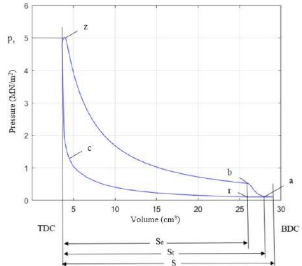
Fig-1: Cylinder -pressure versus cylinder-volume trace for actual cycle
