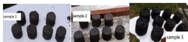
Figure 3: The images of prepared bone char briquettes after sun-drying. Sample 1 has 75% binder, sample 2 has 40% binder while sample 3 has 20% binder.
