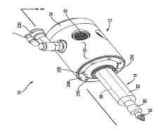
Fig 3: Peumatic Deburring Tool With Articulated Joint
