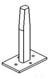
Fig 4: Fixture- Pin Arrangement
