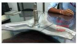
Fig 1: Work piece showing burr forming edges
