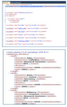
Fig 1: schema and corresponding XML
