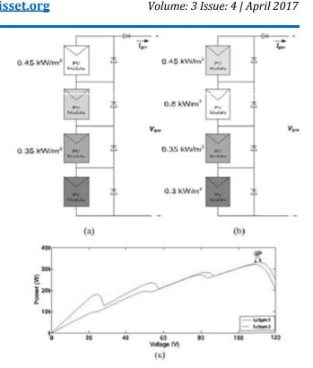
**Fig 1:** 4S configuration under different shading patterns.(a) **P**attern 1(b) Pattern 2.(c) P-V curves **u**nder PSCs.
