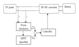
Fig 2: Block diagram of proposed system
