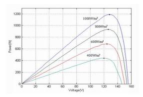
**Fig 3:** PV curve of solar array for different irradiation and constant temperature of 25°C
