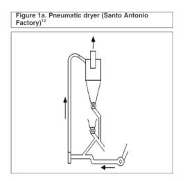
Corrêa et al. 7,8,9 presented theoretical and experimental data on bagasse dry- ing in a cyclone that underwent geometric changes in order to work as a dryer. These authors worked with bagasse with inlet moisture content from 48 to 78% (w.b.); bagasse mass flow in the range of 0.0017 to 0.012 kg/s; GIT 210°C; and air flow rate of 7.8x10-2 kg/s.They succeeded in reducing bagasse moisture content by 74% along
