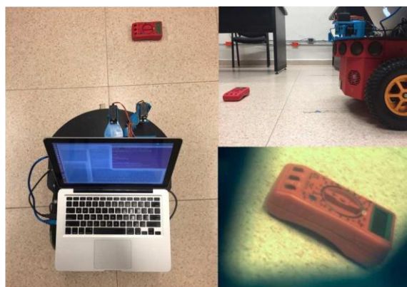
Figure 8: Focusing a visual mark under normal FOV of camera. Left: Top view of the room. Top-Right: Left side view of the robot and the object outside the range of normal view. Bottom-Right: View of the object on the floor, through mirrors.
