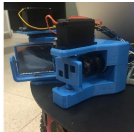
Figure 6: Prototype for ground platform. The system was mounted on the mobile robot and tried to focus on objects outside the normal angle of view of the camera.
