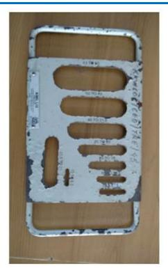
Fig 2: Thickness gauge
