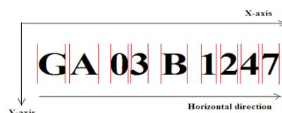
Fig 3: Shows how to implement the algorithm of character segmentation
