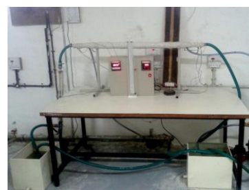
Fig1: Photographic view of experimental set up for forced convection
