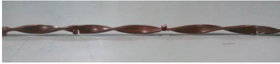
Fig 6: Copper square jagged Twisted tape ( y/w=4 ).
