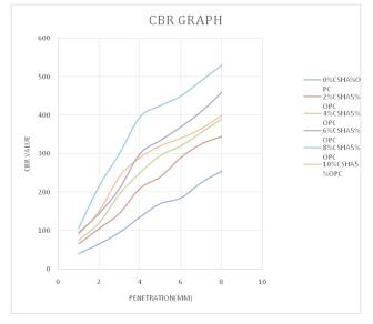
Fig 1: CBR test graph of the effect of CSHA and OPC on studied sample
