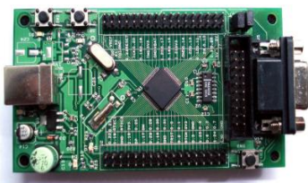
Fig 18: LPC2148 controller board (with ARM 7 processor)
