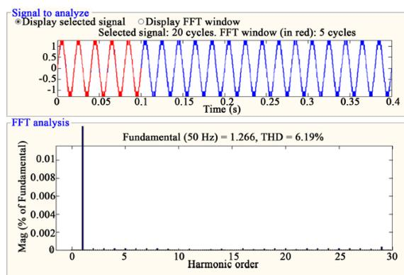
Fig 7: FFT analysis of 13-level inverter with R load for  $M_i = 0.97$  using SHE technique.
