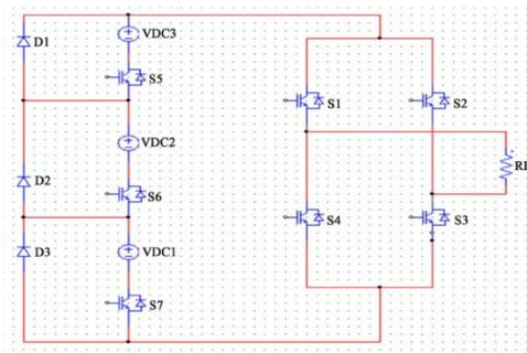
Fig 3: Proposed circuit for Cascaded 13-level Inverter-Asymmetric Topology.
