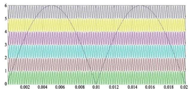
Fig 4: Carrier waveform for SPWM technique.
