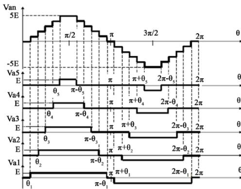
Fig 2: A cascaded 11 level inverter output.
