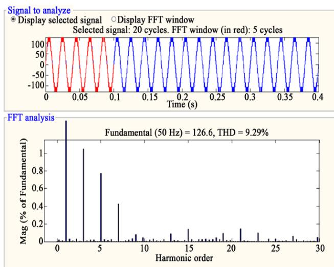
Fig 6: FFT analysis for 13-level inverter with R load.
