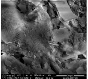
Fig 4: Sample of trepel(microfossil - diatomite)
