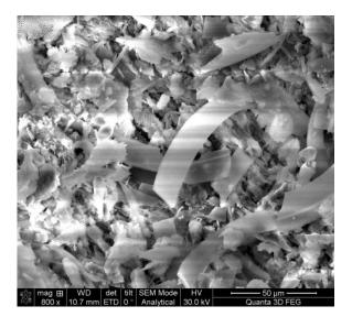
**Fig-3**: SEM-photo of a common trepel mass composed of numerous microrelics – opal globules of biogenetic origin
