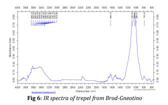
IR spectroscopy is a widely used method when examining amorphous  $SiO_2$ , and especially when studying the way the hydroxyl groups are bonded on the surface of the amorphous  $SiO_2$ .
