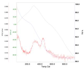
Fig -5: DTA/TGA examinations of trepel
