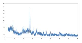
**Fig 2:** X-ray spectra of trepel from Brod-Gneotino (Bitola region), Republic of Macedonia
