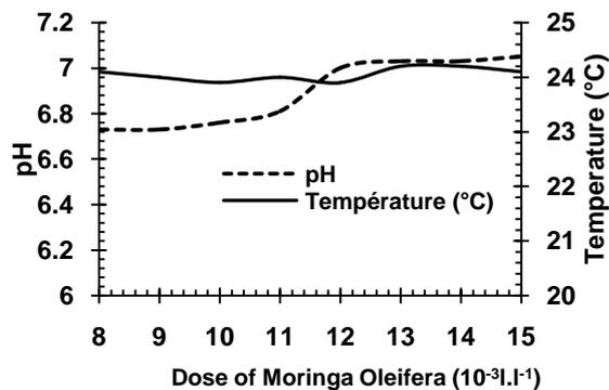
Fig -7: Evolution of pH and temperature with Moringa Oleifera doses
