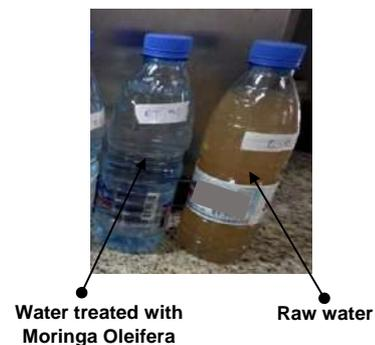
**Fig-6:** Raw water and water treated with Moringa Oleifera coagulant
