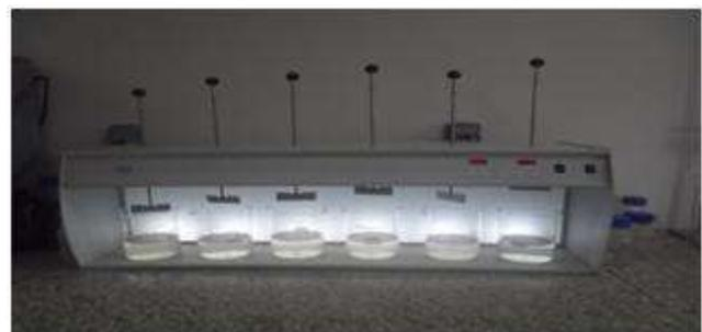
Fig -2: Jar-test flocculator device
