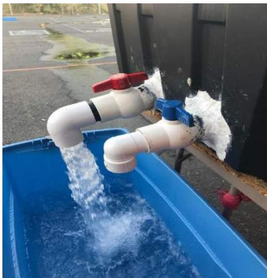
Figure 6: Test run of 2-inch 90° pipe elbow
