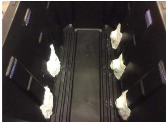
**Figure 4:** Inner tank sealed with epoxy putty
