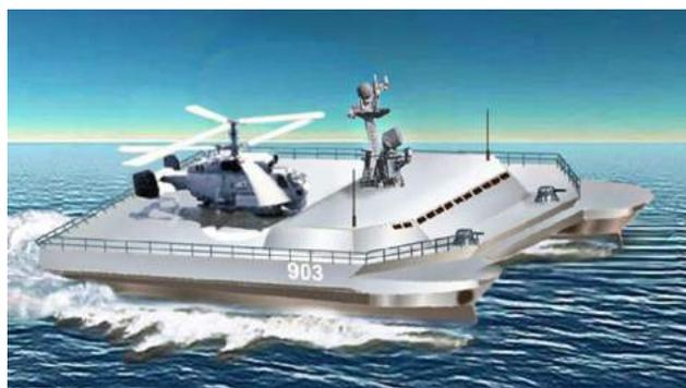
**Fig. 7.** S/P SWA ship as a patrol vessel, the helicopter mass 5 t, deadweight 30 t, 40 knots, Sea State 4 for full
