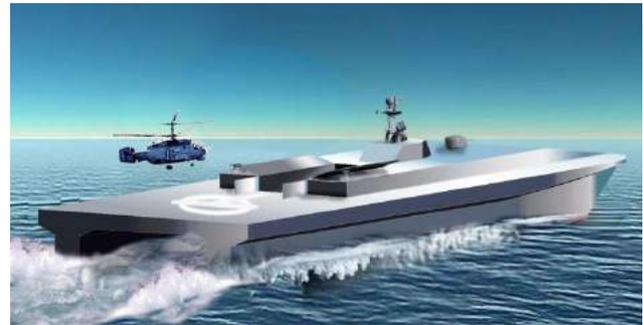
**Fig. 8.** Attack corvette, 400 t, 45 knots, helicopter mass 16 t, Sea State 5 for full operability.
