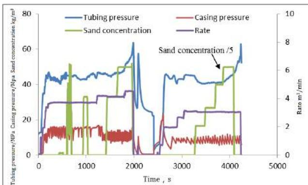
**Fig.1** The fracturing curve of ZH 1-6x well
