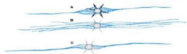
**Fig. 2** Schematic diagram for complex effects and multiple fractures in near-wellbore area
