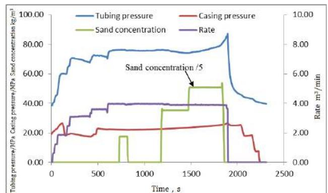
Fig. 8 Fracturing curve of CH 5x well
