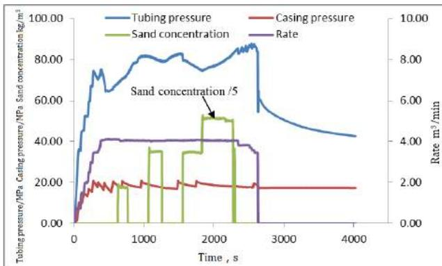
Fig. 6 The fracturing curve of H 129x well
