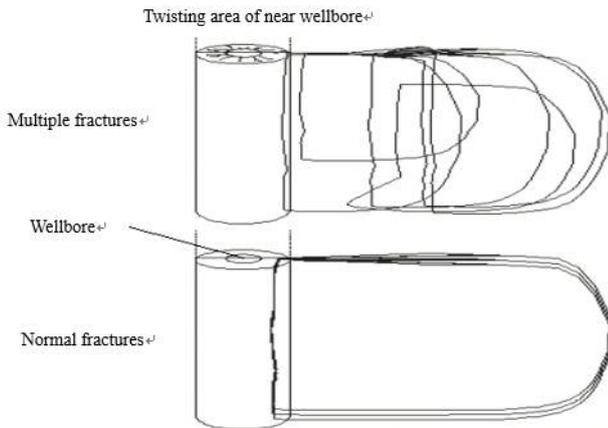
Fig. 3 Normal fractures and multiple fractures
