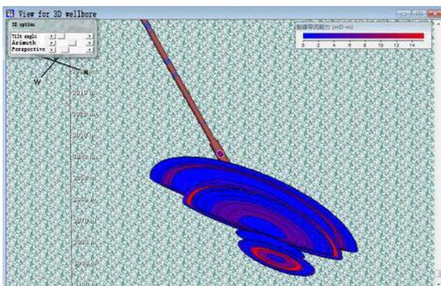
Fig. 4 Fracture profile of L 103-10x well
