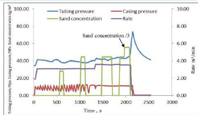
Fig. 5 The fracturing curve of L 103-10x
