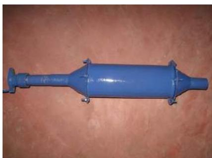
Fig 8: SCR pipe of this project
