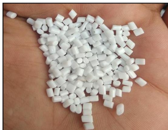
Fig 2: Polyethylene Terephthalate (PET)
