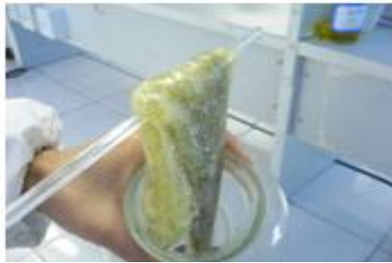
Fig 3: Reaction of marble and cross-linked acid carrying proppant (20 minutes)
