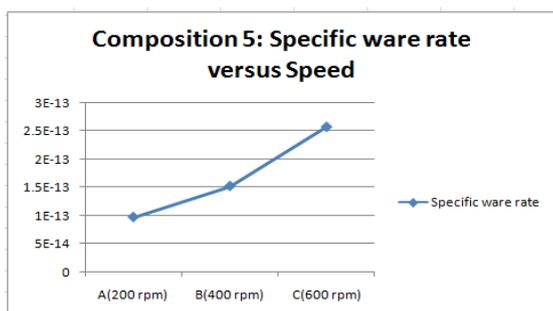
Fig 7: Specific wear rate of composition 5 V/s Speed.
