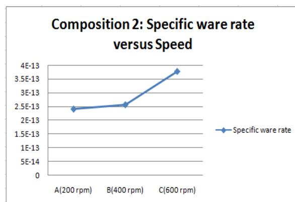
Fig 4: Specific wear rate of composition 2 V/s Speed.
