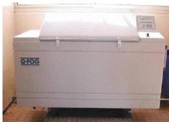
Fig 2: Salt spray chamber
