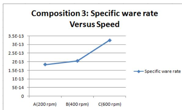
Fig 5: Specific wear rate of composition 3 V/s Speed.
