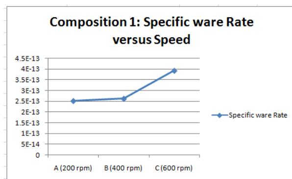
Fig 3: Specific wear rate of composition 1 V/s Speed.
