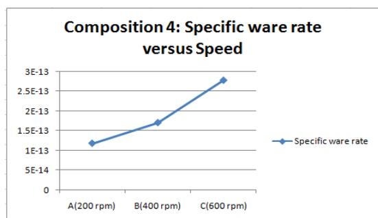
Fig 1: Specific wear rate of composition 4 V/s Speed.
