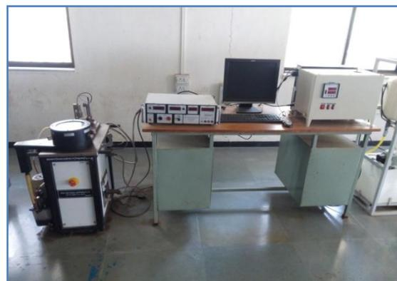
**Fig 1:** Pin on Disc Apparatus
