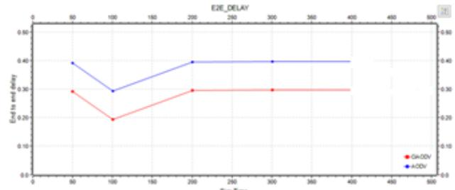
Figure 8: Average End-to-End Delay (ms) Vs Number of cognitive user
