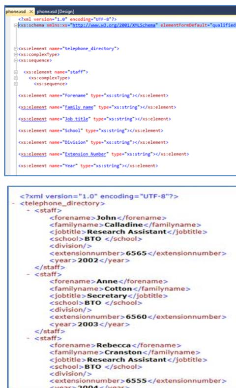
Fig 1: schema and corresponding XML
