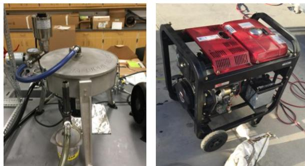
**Exhibit 1:** Centrifuge used to filter WMO. Diesel engine/generator used to test fuels
