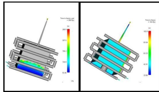
Figure 3: Different types of cooling channels
