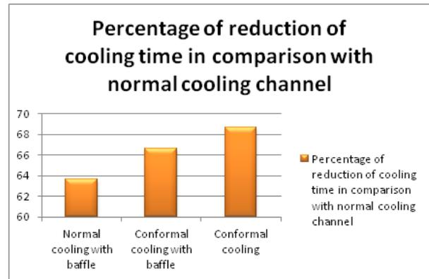
Figure 7: Percentage of reduction of cooling time in comparison with normal cooling channel
