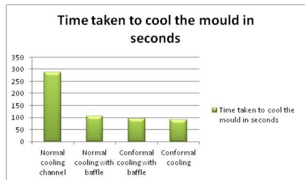
Figure 8: Time taken to cool the component in seconds
