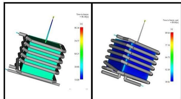
Figure 4: Different types of cooling channels
