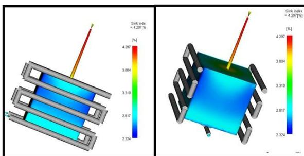
Figure 5: Sink mark on component
