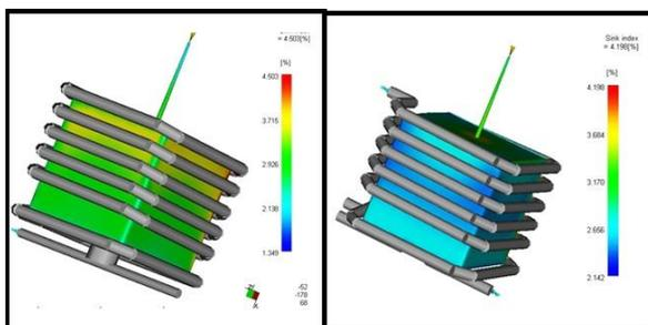
Figure 6: Sink mark on component
