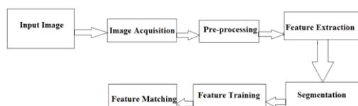
The steps involved in identification of normal and defective quality of Fruits are image acquisition, pre-processing, segmentation, feature extraction, feature training and Feature matching. Finally the quality of fruit is identified.
