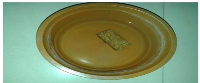
Fig 5: Set-up for Moisture Absorption Test
