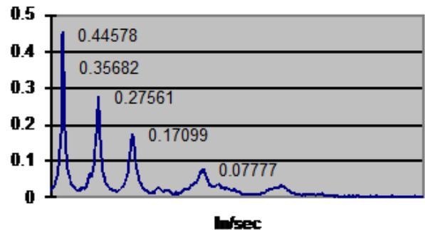
**Figure 6:** Vibration Signature at 1500-RPM using lubricant SAE 90 (Drive end) Unbalance
