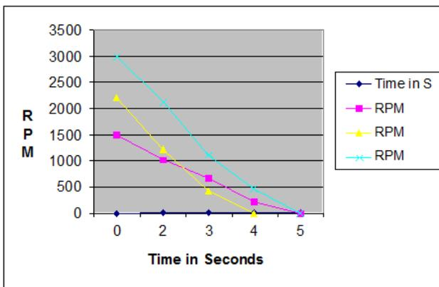
Figure 9: CDT for SAE 90 (Unbalance)
