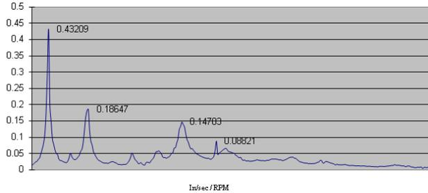
**Figure 2:** Typical Vibration Spectrum at 1500 RPM with SAE 90 lubricant.
