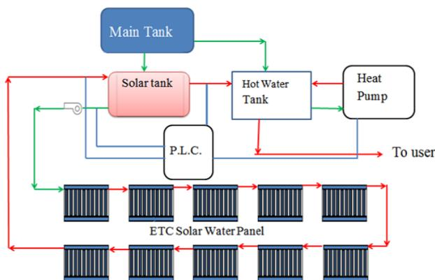
**Figure 1:** Evacuated tube collector integrated with heat pump
