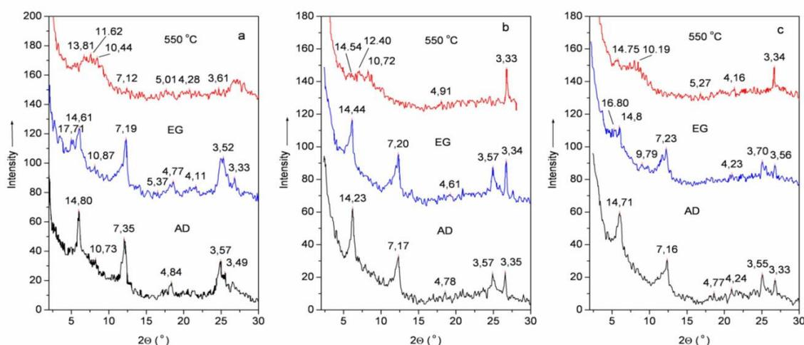
**Fig 4:** X-ray diffractogram of mechanical clay fraction in soil profile 26 Barni Do (a) and profile 29 Babići (b-Amo, c-(B)rz horizon) (AD-air-dried sample, EG- saturated with ethylene-glycol, annealed at 550 °C - 550 °C).
