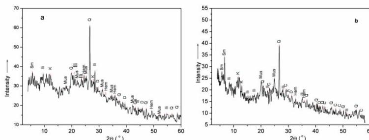
Fig 2: X-ray diffractogram of residuum of geological substrate in soil profile 26 Barni Do (a) and 29 Babići (b)
