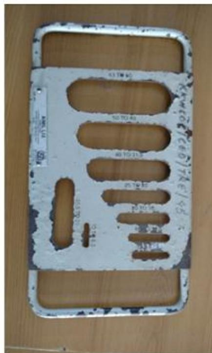
**Fig 2:** Thickness gauge
